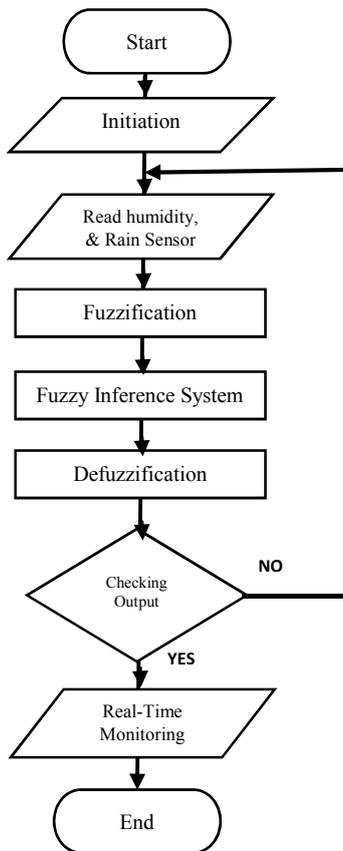
Fig 5. Flowchart Rain Detector
