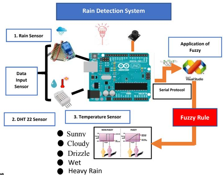
Fig 4. Rain Detector System Architecture
