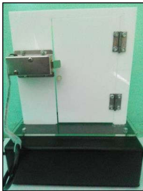
Figure 7. Prototype of Door Automation System
