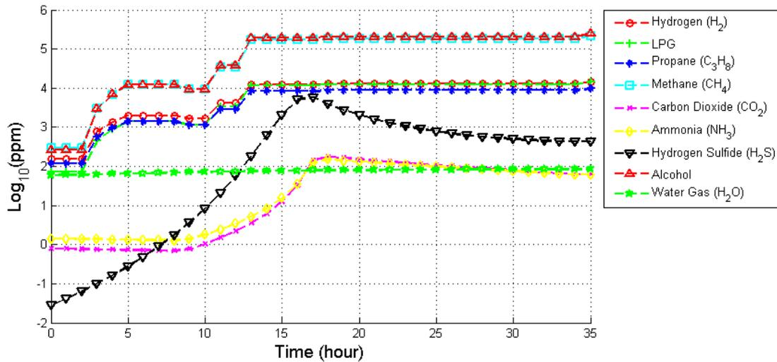
Fig. 9. Various gases concentration (log<sub>10</sub>(ppm)) in beef spoilage
