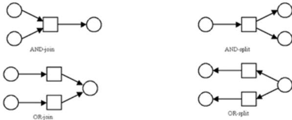
Fig. 1. Type of split and join in petri net
