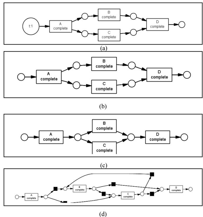
Fig. 4. Result of several discovery algorithm (a) Alpha algorithm (b) Alpha++ algorithm (c) Heuristic algorithm (d) Genetic algorithm
