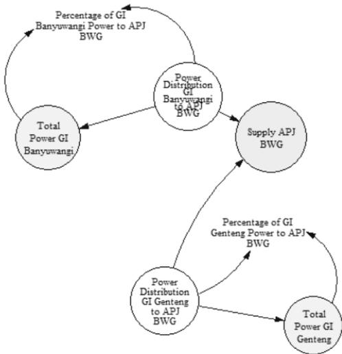
Fig. 4. Electricity Supply SFD.
