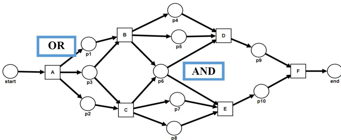
FIGURE 7. Process model of EL II discovered using the proposed algorithm in Petri Net
