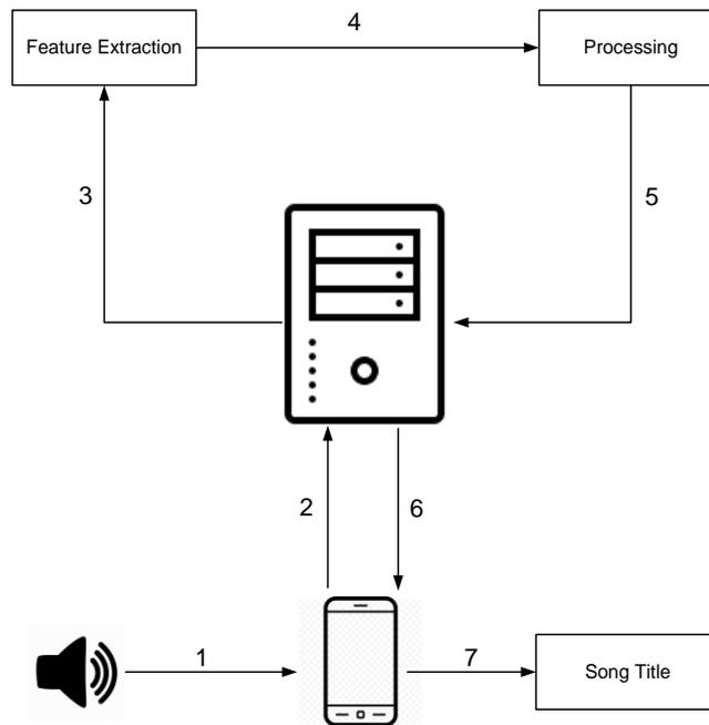
Figure 5. System architecture
