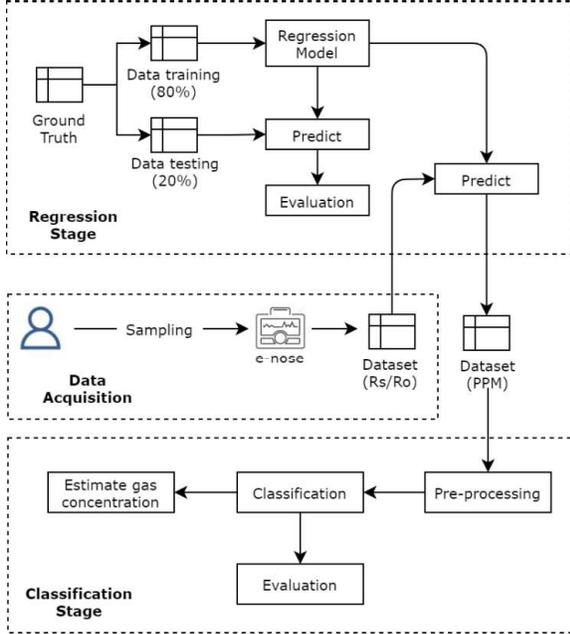
Fig. 2. The scheme of the proposed method
